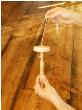
Start by winding a leader around the stem of your spindle, catching it on the notch, and looping through the hook at the top.
