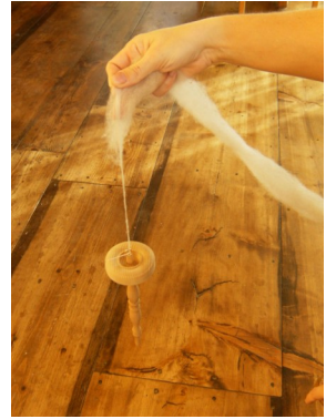
Overlap the fibre in your hand with the end of your leader. Start the spindle twisting, and draft from the fibre in your hand as they overlap and twist into a single strand of yarn.
